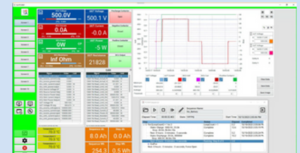
Results display screen showing voltage, current, and the results of a capacity simulation test.
