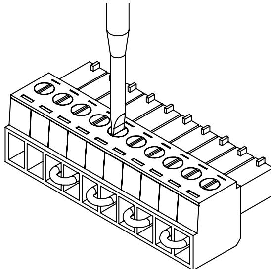
3. Plug the terminal block into the corresponding socket, ensuring it is fully locked in place.
